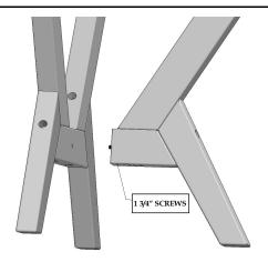
Screw Short Legs into Long Leg and secure from underneath using (2) 1 3/4" Philips head screws.
