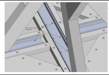
Attach Leg Assembly to Top using (18) 5/8" Pan Head Screws.
