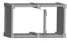
Place Stretcher into pockets in Middle Legs from the bottom of the assembly. Secure using (2) 1 3/4" Phillips Head Screws.
