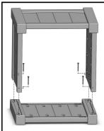
Turn 3-panel assembly over and align End Panels with pockets on Legs of remaining Side Assembly from step 3. Secure using (4) 1 3/4" Phillips Head Screws.
