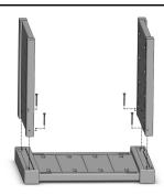
Line up (2) remaining End Panels with pockets on Legs from one of the assemblies from Step 3. Secure using (4) 1 3/4" Phillips Head Screws.
