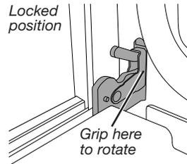
Rotate door hinges from locked to unlocked position.
