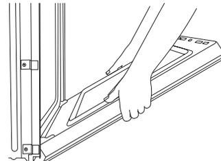
Gently start to close the door. The door will stop at a partially closed position.
