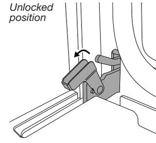
Move door hinges from unlocked to locked position.
