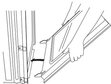
Using two hands, grasp the edges of the oven door. Insert the hinges at the same time and push the oven door into the oven cavity slot to replace. You may need to gently shift door from side to side as you push.
