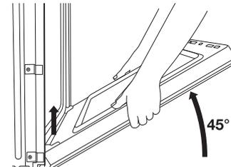
Using two hands, grasp the edges of the oven door. Close the oven door slightly past the stop position to take the weight off of the door hinges and then pull the oven door up.
