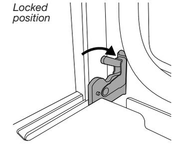
After the door hinges have been locked, gently swing the door upward to close. The door should not be forced closed. Check that the hinges are locked if there is any resistance while closing the door.
