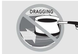
Do not slide cookware across the control or cooktop surface because it can scratch the glass. The glass is scratch-resistant, not scratchproof.
