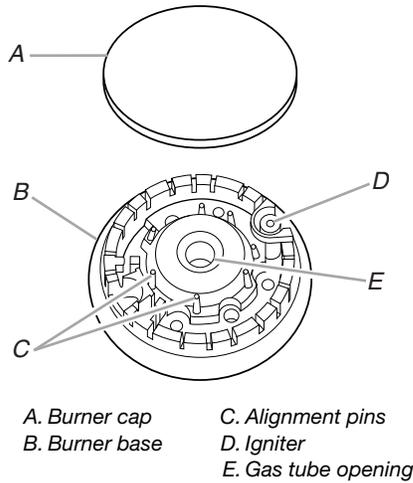
**IMPORTANT:** Do not obstruct the flow of combustion and ventilation air around the burner grate edges.
