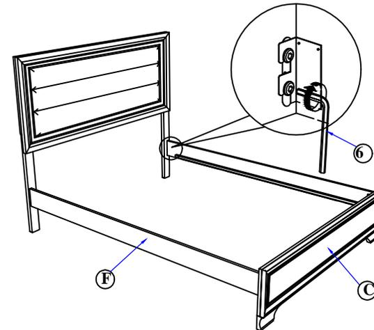
**STEP 3 :** Tighten the 4 Corner with Allen Key ( 6 ). Fix the Bed Slat Support Leg ( E ), to Bed Slat ( D ) as shown . Install the bed slat ( D ) to side rail ( F ) and tighten with Csk Screw ( 5 ) as per diagram shown. ( NOTE: THE SETUP MUST DONE AT THE DECIDED LOCATION FOR THE BED TO OBTAIN PERFECT STABILITY )
