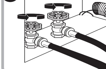
Make sure that the washer is level (see the "Level Washer" section in the Installation Instructions). Run a wash cycle to verify that the washer is working correctly and has no leaks at faucets and inlet hoses.
