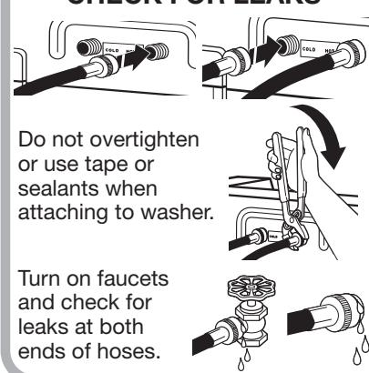
Do not overtighten or use tape or sealants when attaching to washer.
