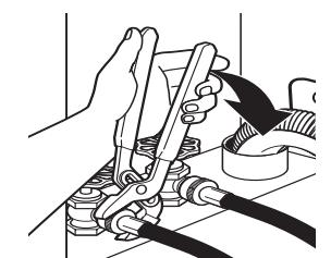
Do not overtighten or use tape or sealants when attaching to faucets.
