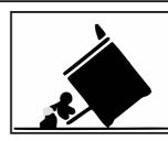
To reduce the risk of tipping the range, the range must be secured by a properly installed **Anti Tip device**. **AFTER THE RANGE HAS BEEN INSTALLED**, **CONFIRM THAT THE ANTI-TIP DEVICE HAS BEEN PROPERLY INSTALLED AND VERIFY THAT THE ANTI TIP DEVICE IS PROPERLY ENGAGED**.
