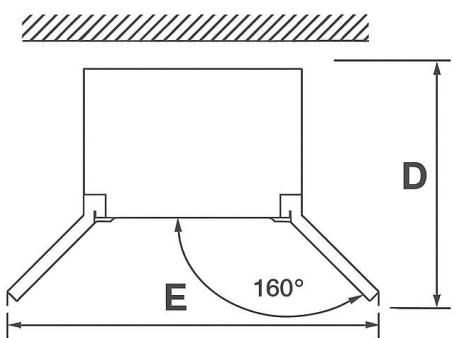
Note: Keep the air circulation free around the cabinet. When installing the unit, leave at least 5 cm (2 in.) of space at the rear of the refrigerator, and ensure sufficient space on both sides and at the top of the refrigerator.
