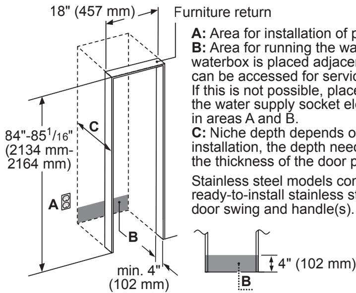
**A:** Area for installation of power connection.
