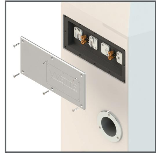
The resistors, located in behind the aluminum plate on the rear of the Yvette, act as an ultra-high-quality fuse which opens before a driver can be damaged by excess power. The midrange and tweeter resistors are attached to heatsinks with Allen hardware.
