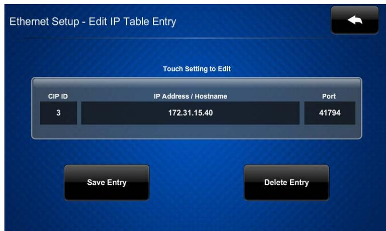
3. Touch the field below **CIP ID** to display the on-screen hex keypad.
