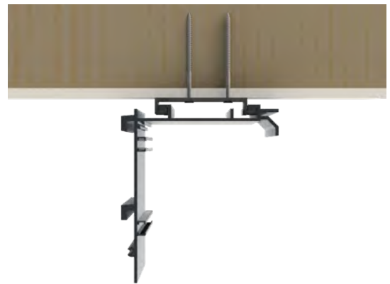
Figure 9. Ceiling bracket screwed onto ceiling joists
