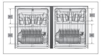
To adjust the Upper Rack position, lift the Adjustment Arms on both sides of the rack and pull up or push down the rack.
