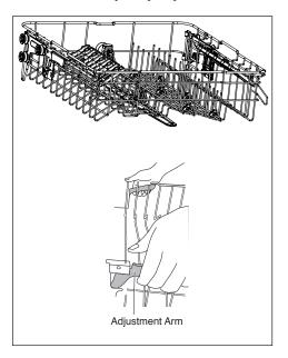
Height should be adjusted without dishes in the racks.
