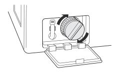
Close the drain pump filter cover.
