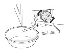
Clean the pump filter and opening.
