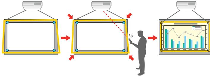
**Note:** The projected image needs to be 100 inches (254 cm) or less diagonally to use the Auto Screen Adjustment. Make sure the projector is squarely facing the projection surface. Auto Screen Adjustment may not work if your image surface:
