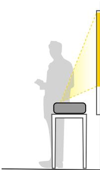
Rear projection from a table or portable cart behind a translucent screen (interactive features not supported)
