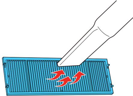
**Note:** If dust is difficult to remove or the air filter is damaged, replace the air filter.
