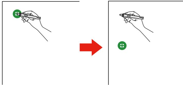
**Note:** For the most accurate calibration, make sure you touch the center of the circle.
