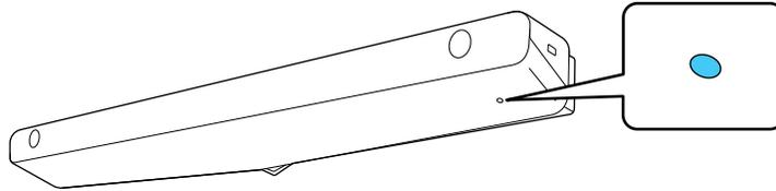
**Note:** If the blue light does not turn on, press the **Menu** button on the remote control and make sure the **Installation > Touch Unit > Power** setting is set to **On**.
