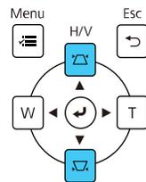
3. Press a keystone button on the projector's control panel to adjust the image shape.
