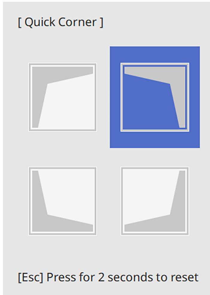
6. Use the arrow buttons on the projector or remote control to select the corner of the image you want to adjust. Then press **Enter**.
