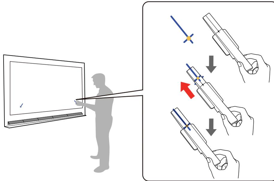
**Note:** If the magnets won't attach to the screen completely, wipe the area to remove any dirt and try again. For non-magnetic screens, use the supplied tape to secure the markers.
