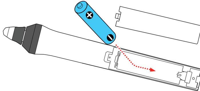
**Warning:** Make sure the batteries are inserted in the correct positions. If the batteries are not inserted correctly, they could explode or leak, causing a fire, injury, or damage to the product.
