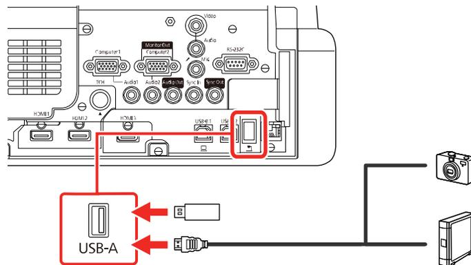
**Note:** Use the USB cable supplied with or specified for use with your device. Do not connect a USB hub or a USB cable longer than 10 feet (3 m), or the device may not operate correctly.
