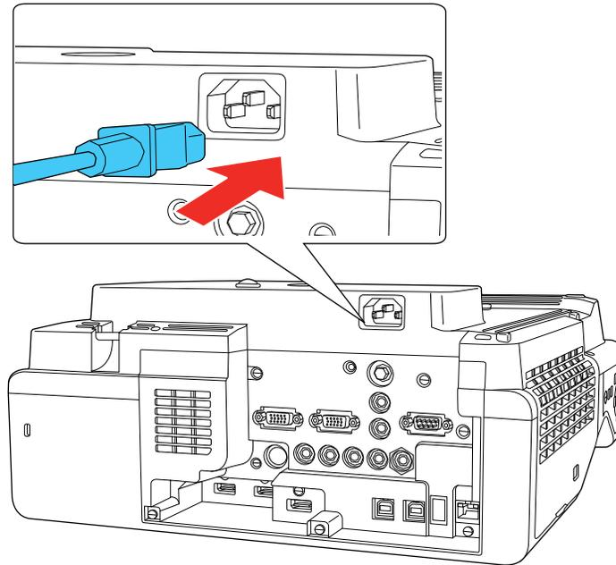
2. Plug the power cord into an electrical outlet.
