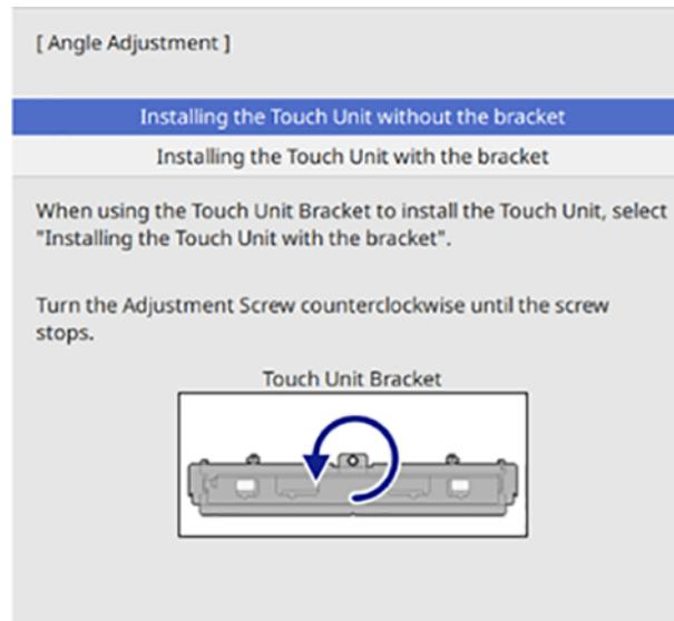
**Note:** The projector automatically detects which touch unit model is connected and displays the instructions for that model. The instructions shown here are for the ELPFT01 touch unit.
