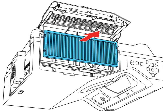
4. Vacuum the front of the air filter (the side with the tabs) to remove any remaining dust.
