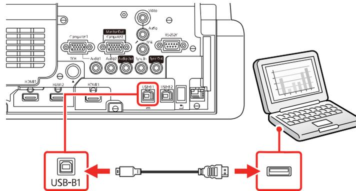
**Note:** If you are connecting to a mini PC attached to the optional wall mount, connect the USB cable to the projector's **USB-B2** port. You can change the HDMI port associated with the USB-B2 port by changing the **USB-B2** setting in the projector's **Pen/Touch > PC Interactivity** menu. Also connect the mini PC to one of the projector's **HDMI** ports.
