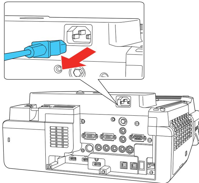
**Caution:** To avoid damaging the projector or laser, never unplug the power cord when the Status light is on or flashing.
