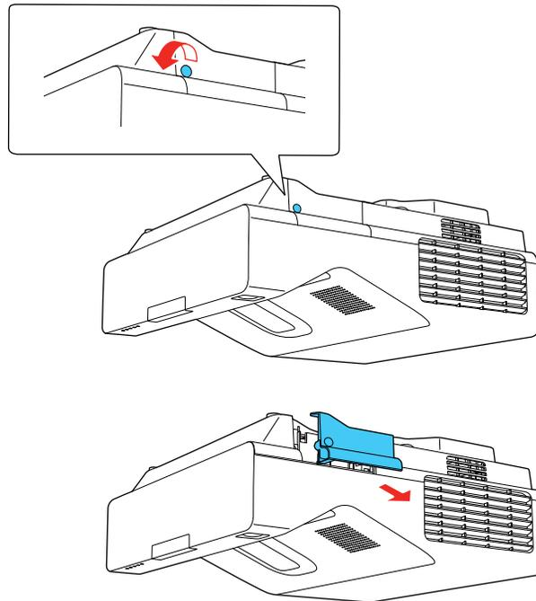
3. Insert the wireless LAN module into the port shown here.
