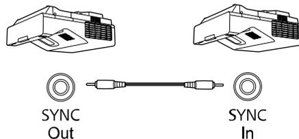
**Note:** If you are connecting three or more projectors, connect the projectors in a chain as shown.
