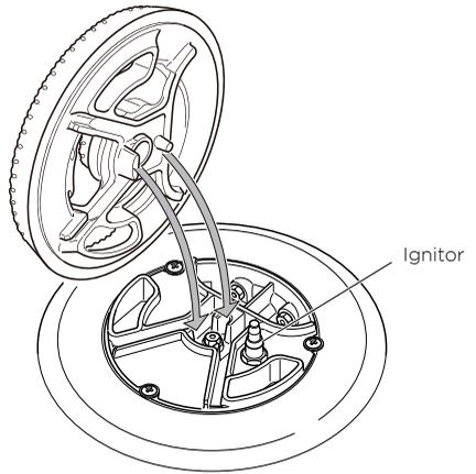
Correct positioning of flame spreader - dual burner
