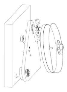
After the placing the record on the platter, it is necessary to tighten the screw-able record clamp (6) onto the platter spindle.
