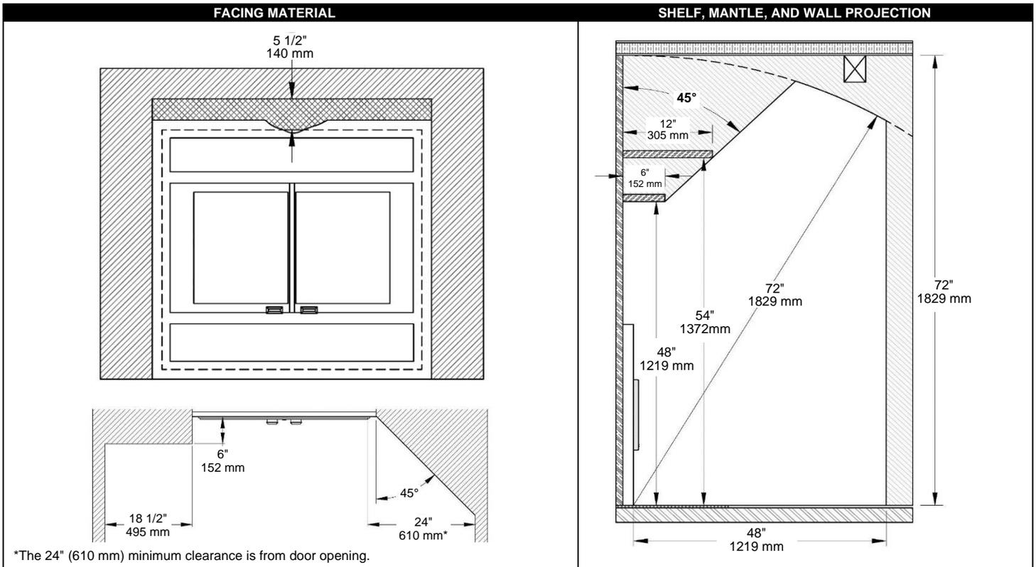
\*The 24" (610 mm) minimum clearance is from door opening.
