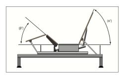
The angle (designated "B" in figure 1) between the flat section and foot section for various configurations of the mattress
