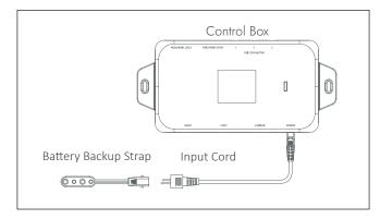
2 Connect the Battery Backup Strap to the (2) 9 Volt Alkaline batteries. Do not mix brand name batteries.
