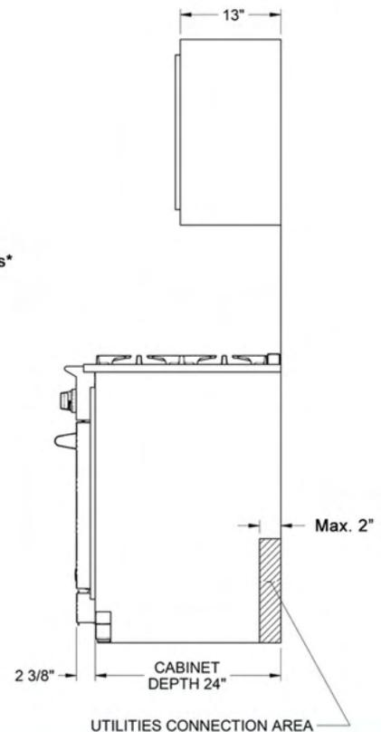
\* For non-ventilation installations clearance to combustable surfaces BSDL60 is 40" min
