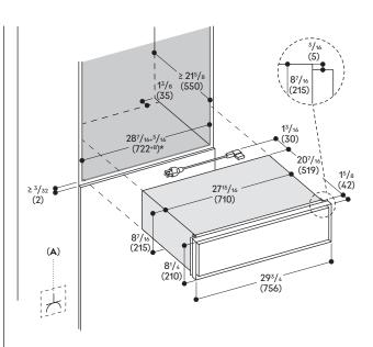
**A:** Accessible electrical connection \* The width tolerance as shown in the drawing indicated by the +  $\frac{5}{10}$ " (+8 mm) is the adjustment possible within the cabinet. Adjustments can be made between  $\frac{5}{8}$ " -  $\frac{13}{16}$ " (16-20 mm) for installation using the "centering parts" within the cabinet for perfect alignment. See installation instructions for details.
