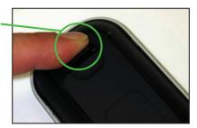
Observe the + and - polarity indications inside the battery compartment.
