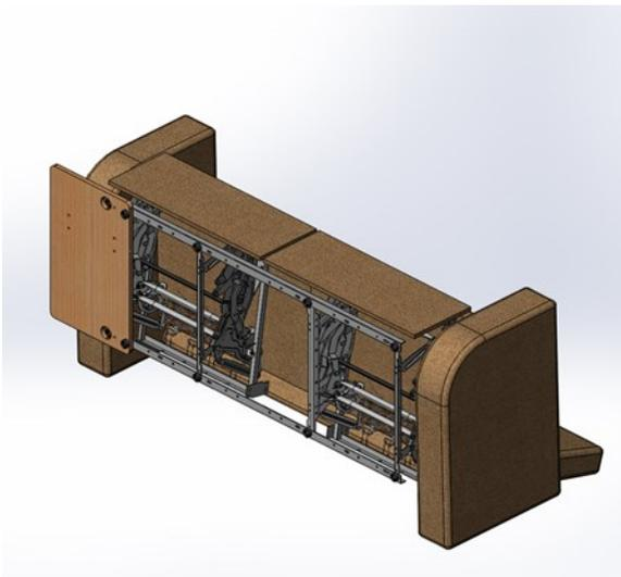
Step 2: Remove two (2) bolts using an 8mm (5/16th inch) socket head and remove cleat.
