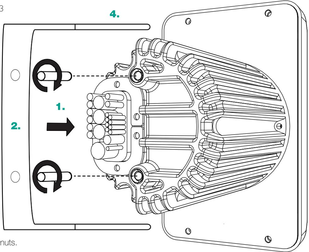
**3.** Place washers over bolts and securely attach nuts.
