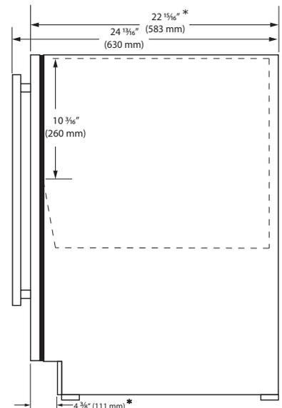
\*Add 1/2" for integrated models with 3/4" panel installed.
