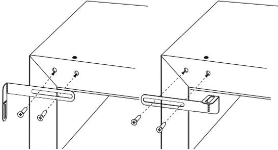
3. Bend bracket along one of the perforations to allow attachment to the desired adjoining surface.
