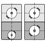
The front and rear elements with two inductors apiece can be used independently. The heat setting is set individually for each element. Use only one piece of cookware on each element.
