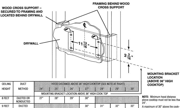
9 FEET **DUCTED** 30" 31" 32" 33" NONDUCTED 27" 28" 29" 30" 31" 32" 33" 10 FEET **DUCTED WITH** 30" 31" 32" 33" RFX6104 FLUE
