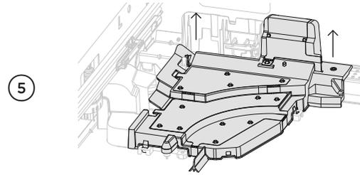
5 Lift the cover upwards until you are able to pull out towards you to remove.
