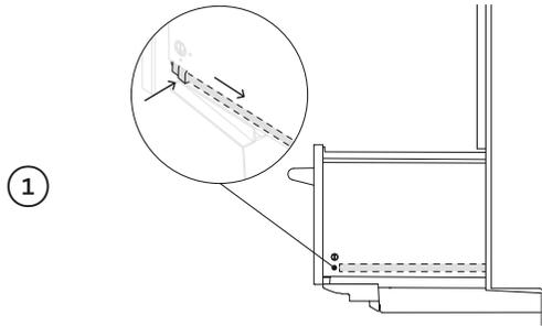
1 Open the lower drawer and press both locking tabs back to release.
