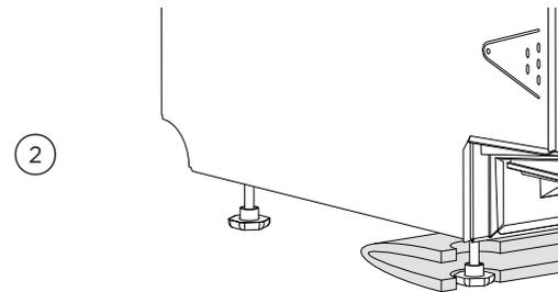
Gently tilt the DishDrawer™ Dishwasher back and align the seal to the front feet.
