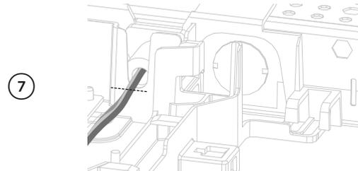
7 Carefully remove the cord from the product. Set toroid aside to for later use.
