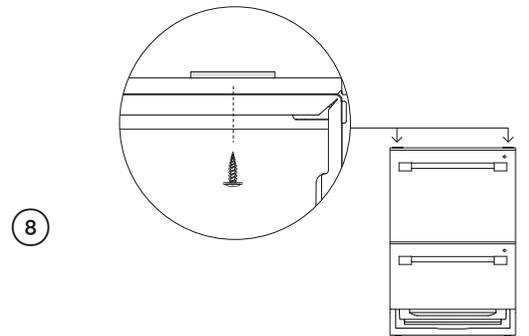
If fitted in step 2, secure the two top brackets to the cabinetry.
