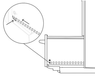
Ensure the hoses are not twisted before refitting the drawer to the runners and clipping into place via both locking tabs.
