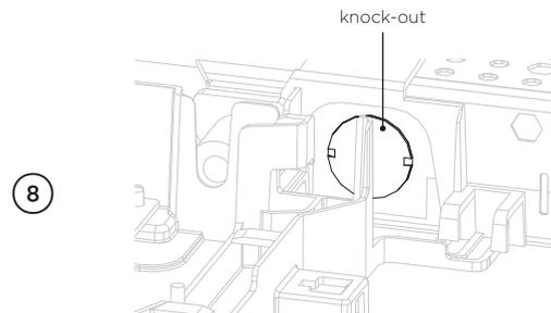
8 Fit a suitable cable clamp for the conduit through the metal knock-out. Route wiring behind the tab and through the toroid removed earlier.
