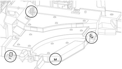
Lock clips back into place by pressing down on the cover firmly. Ensure all illustrated areas are engaged.
