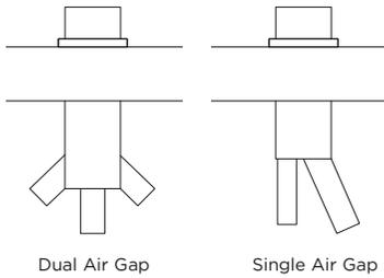
Install your Air Gap Kit to the benchtop. We recommend using a Dual Air Gap Kit. Refer to 'Plumbing & electrical connection' for minimum install heights.
