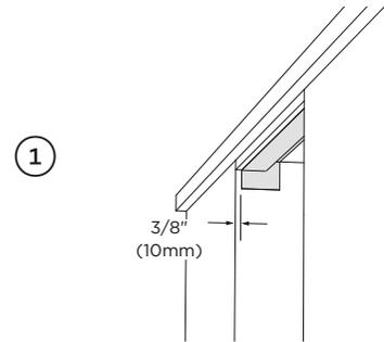
Align the supplied moisture protection tape to the cabinetry as illustrated
