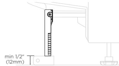
Slide toe kick onto the mounting rails and secure. Ensure a 12mm clearance is maintained between the floor and the toe kick, the end tabs can be used to measure this if desired.
