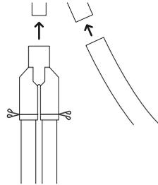
Thread wire clips onto the hoses before fitting them to the hose joiner. Secure using the wire clips. Fit the joiner to the Air Gap Kit and secure using the hose clamp. Ensure hoses are routed straight to the joiner, removing excess drain hose if necessary.
