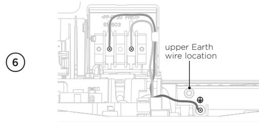
6 Unscrew the Live, Neutral and Earth wires as illustrated. **Ensure the upper Earth wire is not removed.**
