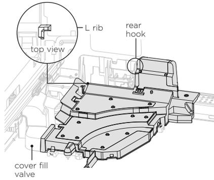
Position the cover fill valve into place before lowering the rest of the cover into position.
