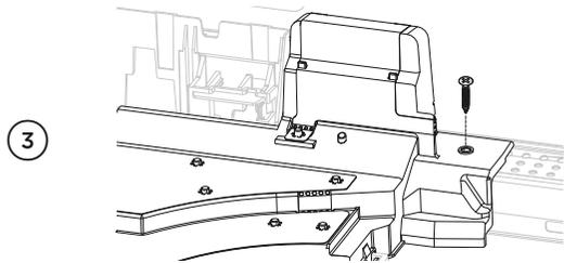
3 Remove the screw securing the cover. Set aside.
