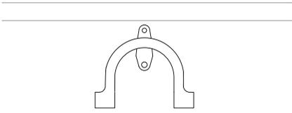
Install the drain hose support to the back wall, as close to the underside of the countertop as possible. Refer to 'Plumbing & electrical considerations' for minimum install heights.
