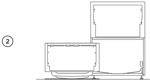
2 Lift the drawer off the runners and carefully set aside on a protected surface. Push runners back in. Take care not to pull drawer out too far to prevent any strain on the hoses. Where possible, protect the base of the tub to prevent damage.
