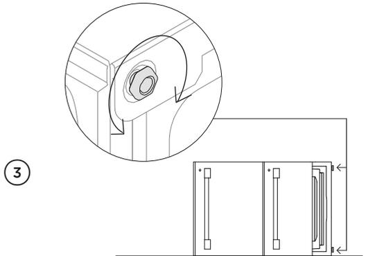
Level the DishDrawer™ Dishwasher by carefully tipping it onto protected surface.
