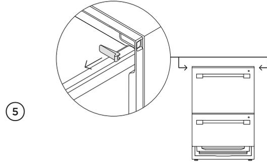
Partially open one of the drawers and remove the first screw cover from the trim moulding.
