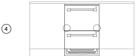
Push the product into the cavity, pulling the hoses through as you push to avoid crushing or twisting them and taking care not to bend the legs.
