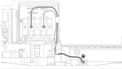
Fix the Live and Neutral wires to the terminal block and the Earth wire to the chassis.
