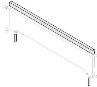
Snap off excess toe kick material and both end tabs.
