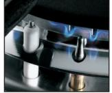
All Foster cooker hobs are equipped with safety valves. These shut off the gas supply very quickly if the flame accidentally goes out. The utmost freedom of movement it is guaranteed by the electronic under knob ignition that allows
