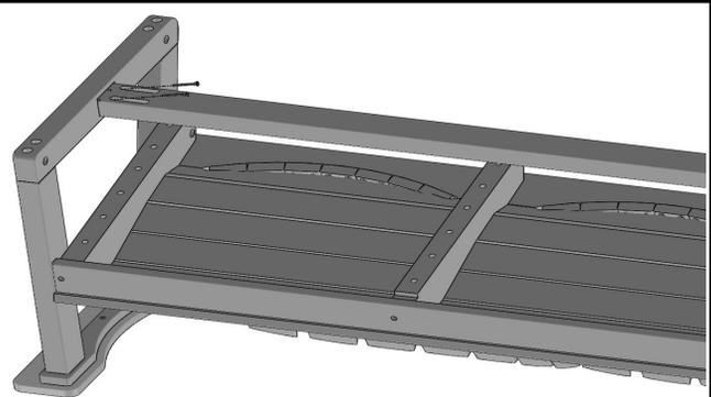
Align Short Stretcher with notch in Side Assembly. Secure using (4) 1-3/4" Phillips Head Screws thru pre-drilled holes in stretcher.
