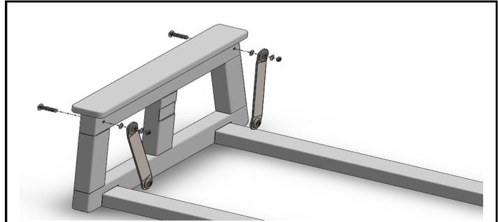
Secure Bearing Straps to Base Assembly using (2) 1-1/2" Phillips Pan Head screws (4) 5/16" Flat washers (1 before and 1 after bearing strap)\* and (2) 5/16" Lock Nuts with a #3 Phillips Screwdriver and a 1/2" Wrench. Plug holes in base with (2) 5/8" plugs.
