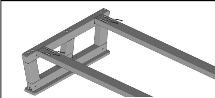
Align (2) Long Stretchers with the notches in the lower leg of the Base Side. Secure using (4) 1-3/4" Phillips Head Screws.
