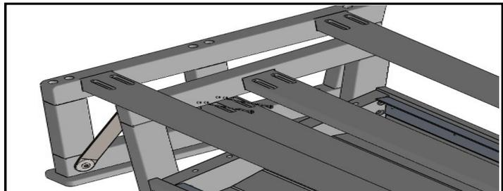
With Glider upside down, rock the base so that the notch in the middle upright is accessible. Attach long stretcher to base using (2) 1-3/4" Phillips Head Screws.
