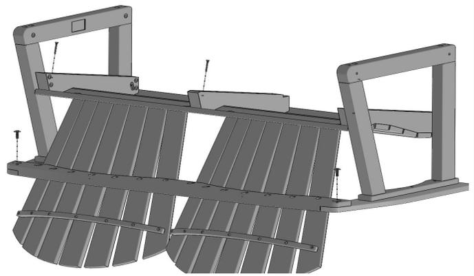
Align Back Assembly with seat supports and arms. Attach using (3) 1-3/4" Phillips Head Screws thru Seat Supports into Lower yoke of Back Assembly, and (2) 1" Phillips Pan Head Screws from upper yoke into threaded inserts in arms.
