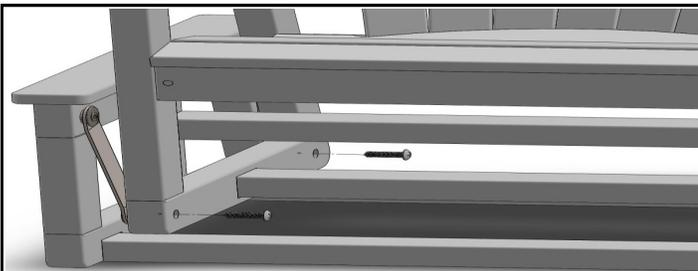
Secure Bearing Straps to Seat Assembly using (2) 1-1/2" Phillips Pan Head screws (4) 5/16" Flat washers (1 before and 1 after bearing strap)\* and (2) 5/16" Lock Nuts with a #3 Phillips Screwdriver and a 1/2" Wrench. Plug holes in legs with (2) 5/8" plugs.
