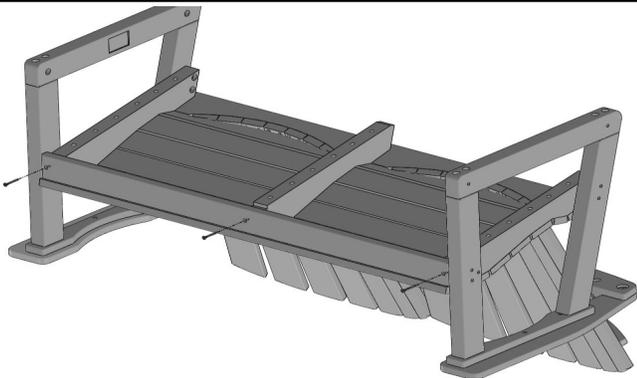
Align Aluminum on Apron with the notch in the middle seat support (016 only). Attach Apron to front of seat using (3) 1-3/4" Phillips Head Screws (2 for 116). Plug holes with 3/8" Bungs.
