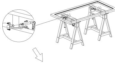
STEP 2: WITH PINS REMOVED, RAISE TABLE TOP TO DESIRED HEIGHT AND REINSERT PINS.
