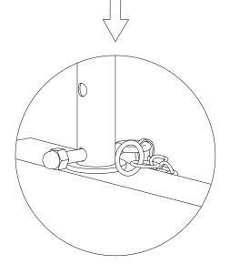
STEP 3: ENSURE THAT PINS ARE SECURED TO PREVENT ACCIDENTAL REMOVAL.
