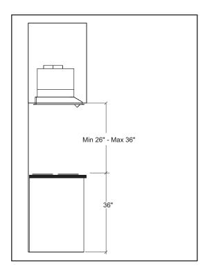
Minimum mount height between range top to hood bottom should be no less than 26".
