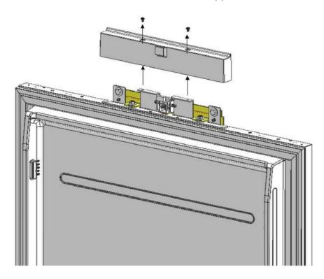
Note: There is a magnet in the cover of the top refrigerator door hanger bracket. This is a functional part for the operation of the product.
