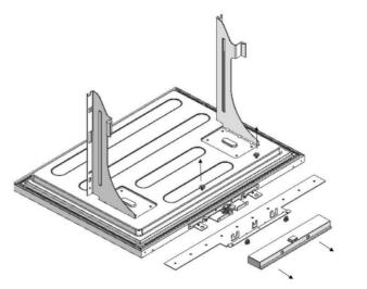
You must take the dimensions into account when grouping the door panel brackets on the door panels. When marking, you can use the "Door panel preparation template" (Item No 6) provided with the product.
