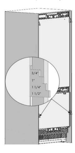
Position of the position alignment gauge (10) must be adjusted according to the thickness of the door. It can adjust the level for 4 different door thickness levels.
