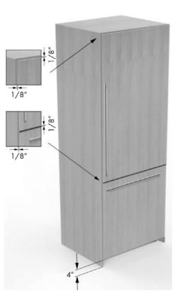
After carefully pushing the product into the cabinet, the feet need to be raised in order to secure the product to the anti-tip brackets.
