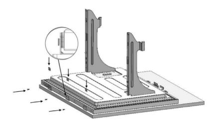
A total of (3)1 mm washers must be placed on the freezer door on the condition that all door panel dimensions are suitable. Washers to be used are determined based on the kitchen design.
