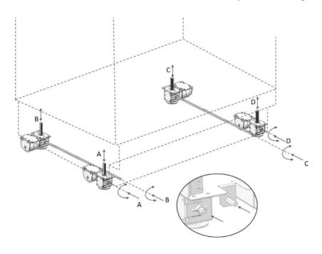
A/D -Turn the key clockwise to lift the front B/C –Turn the key clockwise to lift the rear
