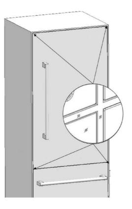
For products without clad doors, the product is placed using the position alignment gauge (Item No 10) as shown in the figure below.
