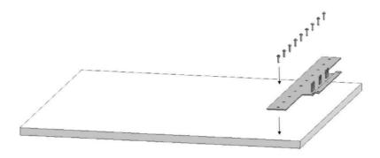
• Attach 3 sheet metal brackets (Item No25) using 6 screws (Item No 15) for each.
