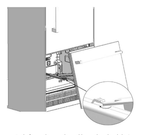
• Fix the freezer door panel assembly onto the rails with the 2 screws removed earlier.
