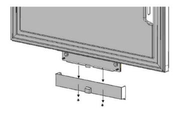
Remove lower and upper bracket screws.
