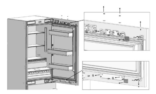
• Remove the screw of upper and lower mechanisms.
