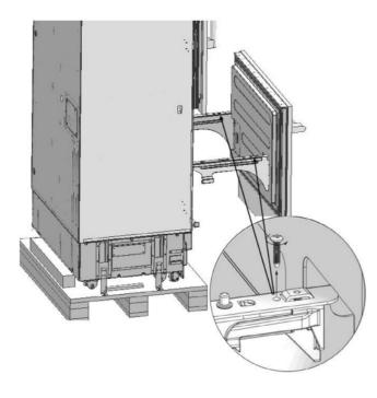
While supporting the door, pull it forward while freeing it from the rear rail lock tabs to remove it.
