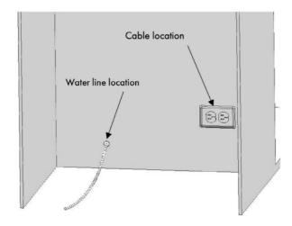
• Method B: Locate the water hose and power supply on the back
