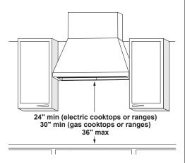
For this installation, conceal the ductwork running from the top of the hood. Use of the duct cover requires special consideration to the installation height above the countertop.
