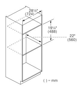
NOTICE: The cabinet base must be flat and capable of supporting a weight of at least 142 lbs (64.1 kg).
