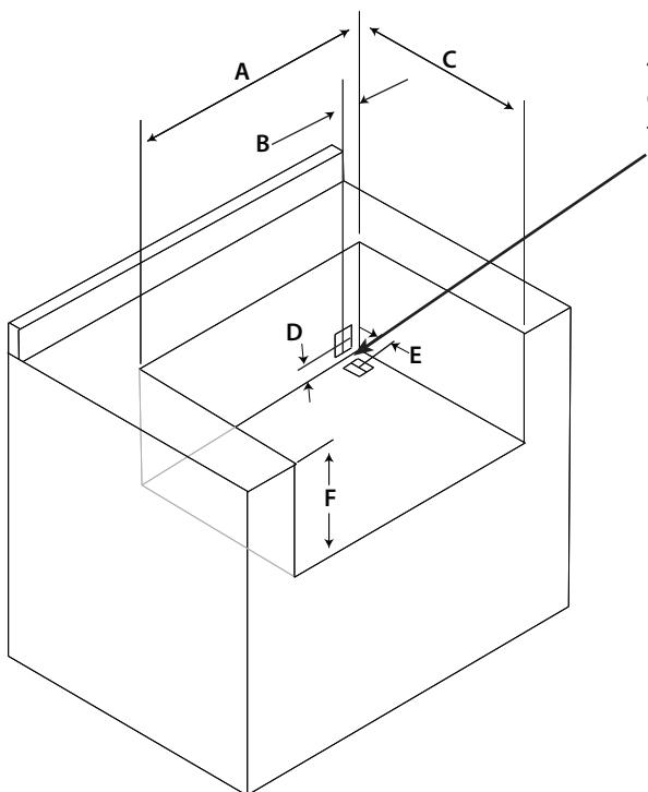
4" square holes for gas and electrical connections (rear or bottom access). Make these holes in the frame based on your requirements
