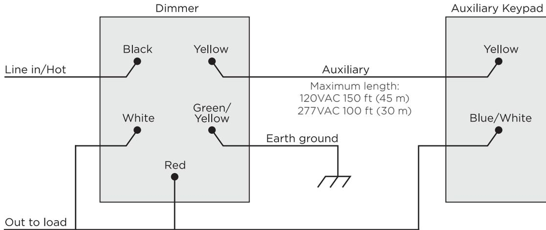
**IMPORTANT!** When used in conjunction with an Auxiliary Keypad (C4-KA-xx), the wire connecting the Auxiliary Keypad to the dimmer must not exceed 150 feet (45 m) at 120VAC, and 100 feet (30 m) at 277VAC.
