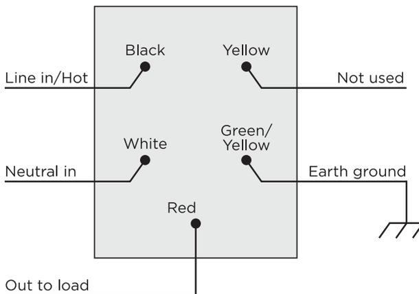
Figure 5. Single device location, without neutral connection
