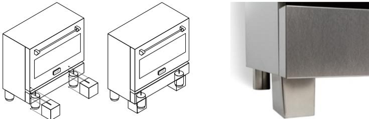
**NOTE:** If the range is not level, the cooking will be uneven. When adjusting the legs, ensure they are the same height.
