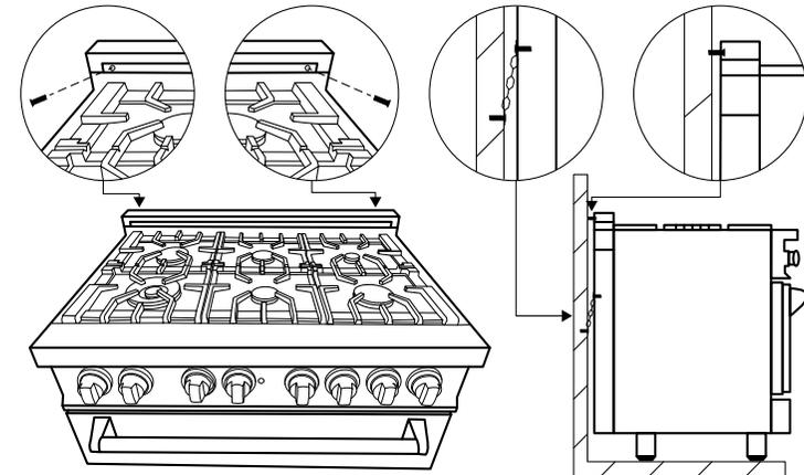
1. Measure the distance from the floor to the where the chains connect on the back of the appliance.
