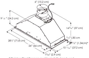
\* Stainless Steel Spacers must be installed and used when cabinet depth is greater than 12"
