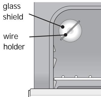
Figure 37: Oven light protected by glass shield
