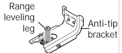
To check if the anti-tip bracket is installed properly, use both arms to grasp the rear edge of the range back. Carefully attempt to tilt range forward. When properly installed, the range should not tilt forward.
