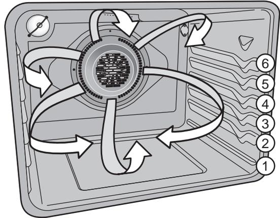
Figure 23: Convection roasting on lower oven racks
