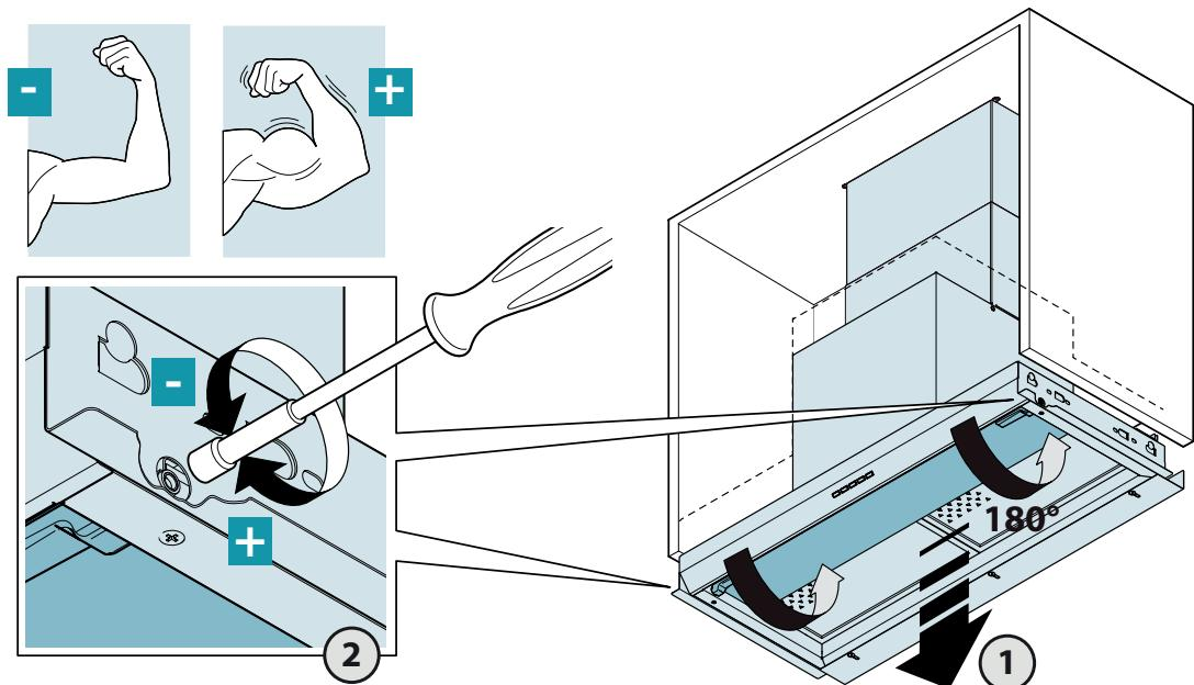
EN - Assembling standard active carbon filter: , remove metal filters (8), assemble active carbon filters (9).
