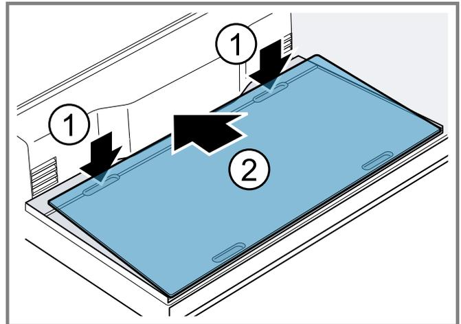
2. Grip both the front recesses at the base of the refrigerator compartment ①, lift the refrigerator compartment glass plate and remove it ②.
