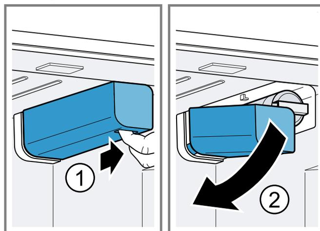
2. Turn the water filter counterclockwise by 90° ① and remove it ②.
