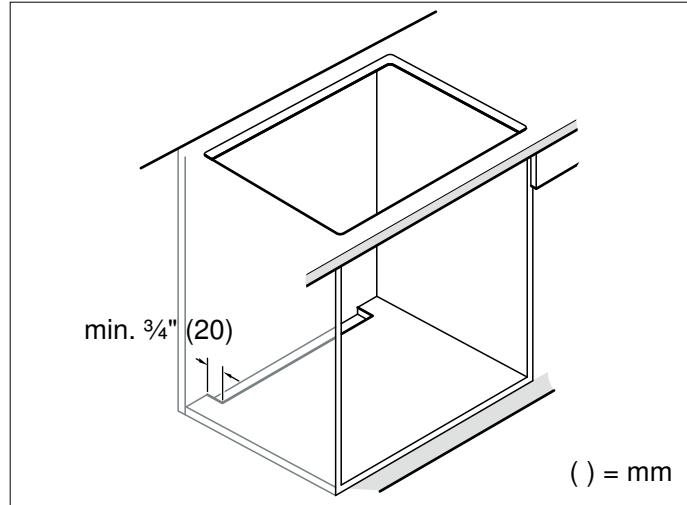
**Note:** If the appliance is installed in an island unit or another installation that is not described here, you must ensure that the cooktop is sufficiently ventilated.
