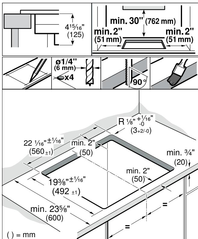
**Combining several Vario appliances:** Consider additional space requirement for the connecting strip VV 200 when making the cut-out. Appliances can also be installed in individual cut-outs, if a minimum clearance of 1½" (40 mm) between the appliances is observed.
