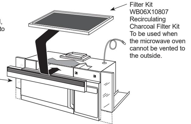
**Filter Kit WB06X10807 Recirculating Charcoal Filter Kit**
