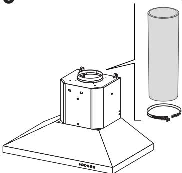
Only for the recirculation version, connect the hood to the Air outlet.
