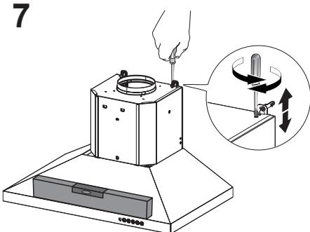
Use a level to insure that hood body is level and then fully secure the two screws.
