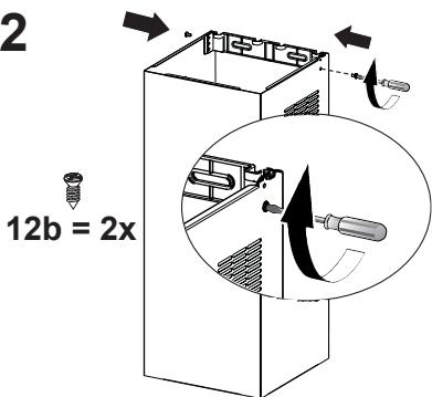
Secure the sides to the brackets by using the 2 screws 12b.
