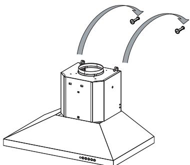
Hook the hood body onto the hood body fixing screws.
