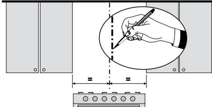
Draw a vertical line on the supporting wall as high as practical, at the center of the area in which the hood will be installed.
