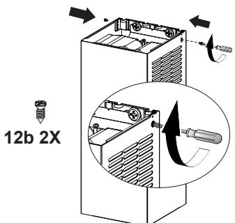
Secure the sides to the brackets by using the 2 screws 12b.
