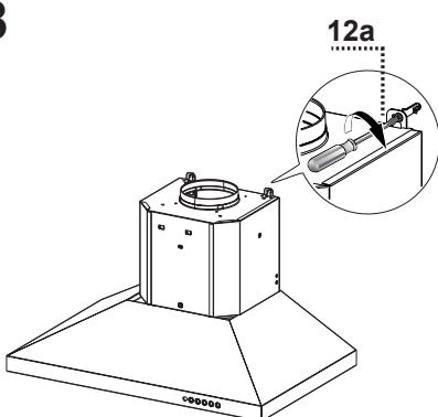
Tighten the 2 screws 12a as shown.
