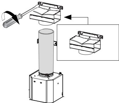
Fix the Ductless Diverter with two screws 12a supplied as shown.
