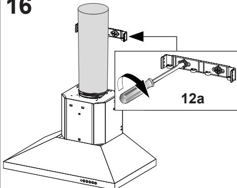
Fix the lower Bracket 7.2.1 with two screws 12a supplied as shown.
