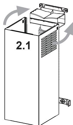
Slightly widen the two sides of the upper chimney and hook them behind the brackets and connect to the Ductless Diverter, making sure that they are well seated.
