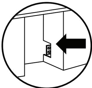
TIP: IN TIGHT INSTALLATIONS CUT THROUGH AN ADJACENT CABINET WALL TO REACH AN OUTLET INSTALLED THERE
