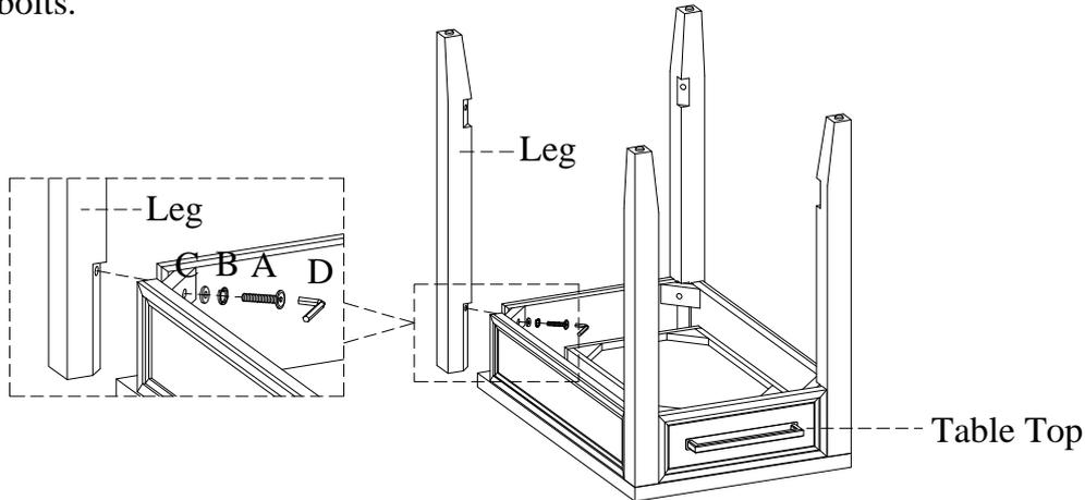
**STEP 2:** Attach the shelf frame to legs by using 4 bolts(A), lock washers(B), flat washers(C) with an allen wrenches(D). Completely tighten all bolts. Turn the assembled table to the upright position.
