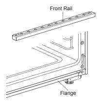
**3** Use the 3 screws provided to secure the front rail to the flange.
