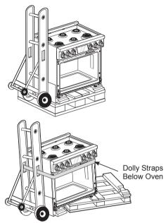
**4** Transport the range on the furniture dolly close to its final location, tip the range back to level, and carefully remove the dolly.
