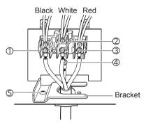
After removing the bracket and power cord, use the cord/conduit connection plate enclosed in the accessory box to install the power cord or conduit.
