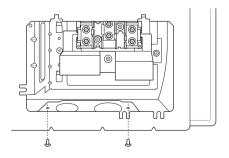
For power cord installations, hook the strain relief over the  $1^{3}/_{8}$  in. (3.5 cm) power cord hole located below the rear of the oven. Insert the power cord through the strain relief and tighten it.
