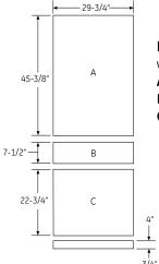
\*Styles must be a min  $3^{3/4}$ " to cover aluminum door frame. **Design Tip:** Some amount of each panel will be visible on the interior side of the unit. It is recommended that both sides of each panel be finished.
